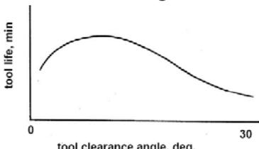
Inadequate clearance angle reduces tool life and surface finish by tool - work rubbing, and again too large clearance reduces the tool strength and tool life hence machinability.
